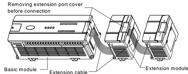
Figure 1-3 Connecting into system
