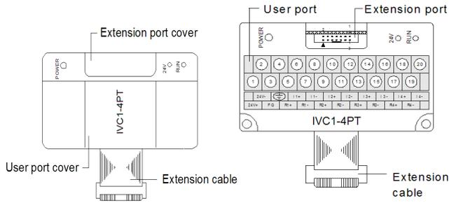
Figure 1-1 IVC1-4PT appearance Figure 1-2 IVC1-4PT ports
